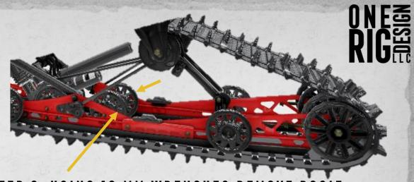
STEP 2: USING 10 MM WRENCHES REMOVE BOGIE INSIDE BOGIE WHEELS MARKED ABOVE.
